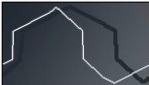
The **oscilloscopes** let you see what is going on. There is one for each **oscillator**, and one for the main **output**. The light line represents the left signal and the dark line represents the right signal.
