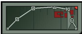
The **envelope** module is an **envelope** generator just like the ones in each **oscillator** module, except that it produces a **modulator** signal that can be used on any of the **sliders**. When a **note on** event occurs, the envelope starts, and loops between the loop points until a **note off** event occurs, at which point the release begins. At release, the volume fades to the release value and then follows the envelope normally.
