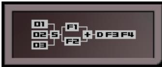
**Atlantis** can perform the **filtering** and **waveshaping** functions in a variety of different ways so you can create all kinds of sounds. The routing window displays the current order of operations. The signal flows from left to right. In the above image, the **routing** is set so that the **oscillators** feed into the **shaper** and then the signal is split and fed **parallel** into the **filters**, which are **added** back together before flowing into the **delay unit**.
