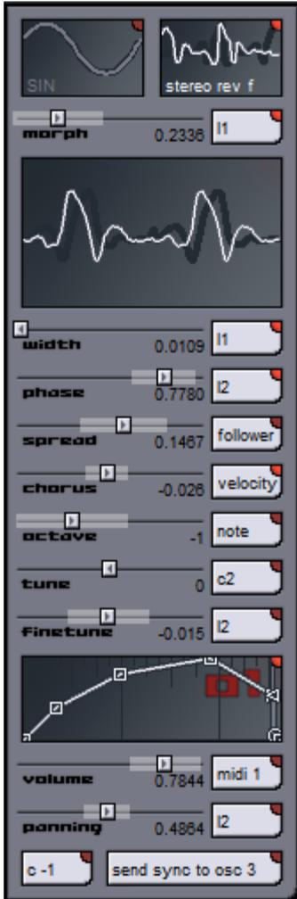
**Oscillators** are where the sound is generated. A number of parameters can be adjusted to control the way in which it is generated before it is passed on to the **filters, shaper** and **delay**.
